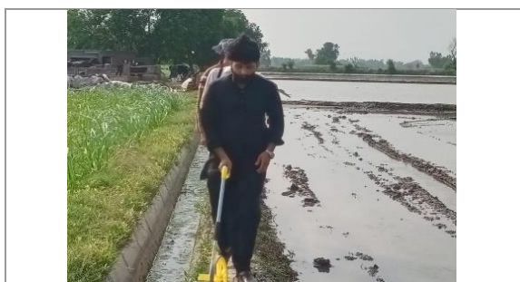
Figure 4.61: Measuring the Length of watercourse with measuring wheel of Watercourse No 58622/TL
