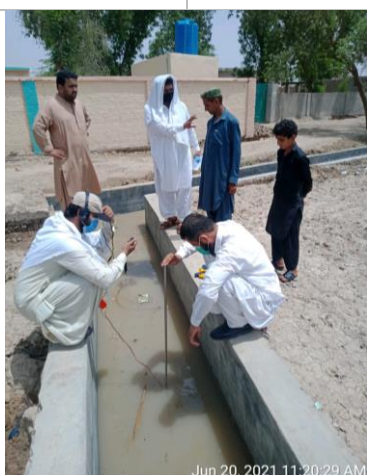
Figure 4.93: Checking Water flow using Pygmy Meter
