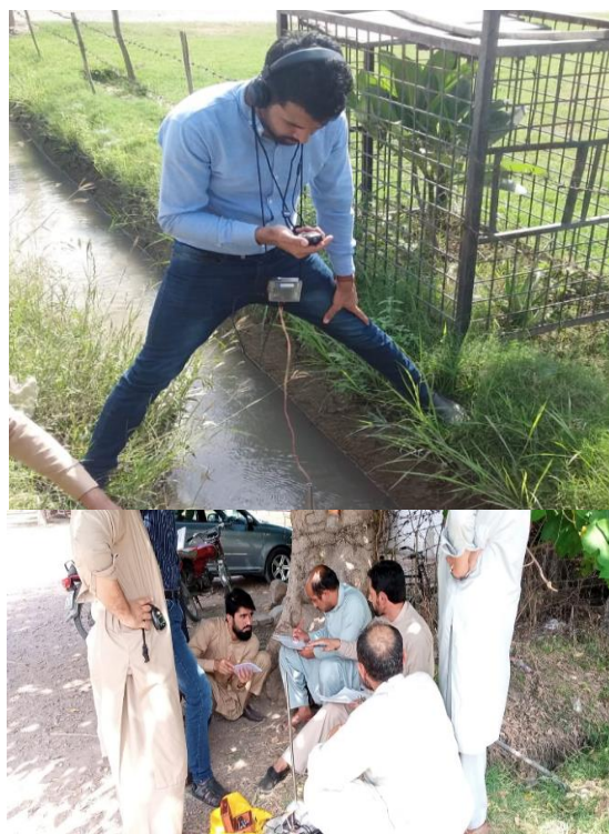
Figure 4.4: During Training Field Team Engineers performing water flow measurement by pigmy meter on a watercourse.
