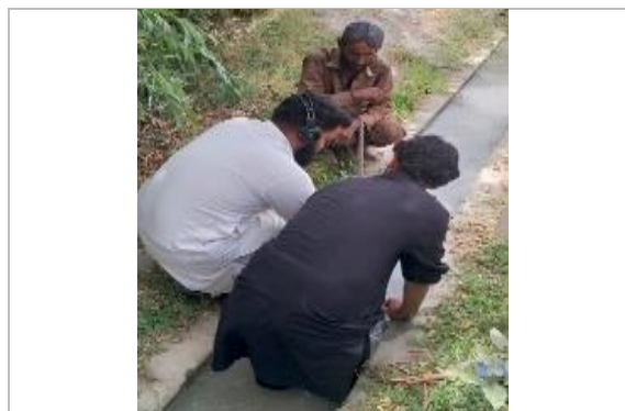
Picture 3.31: Measurement of Discharge by Pygmy Meter at WC No. 26750/L
