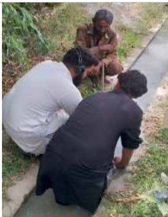
Picture 4.77: Measurement of Discharge by Pygmy Meter at WC No. 26750/L
