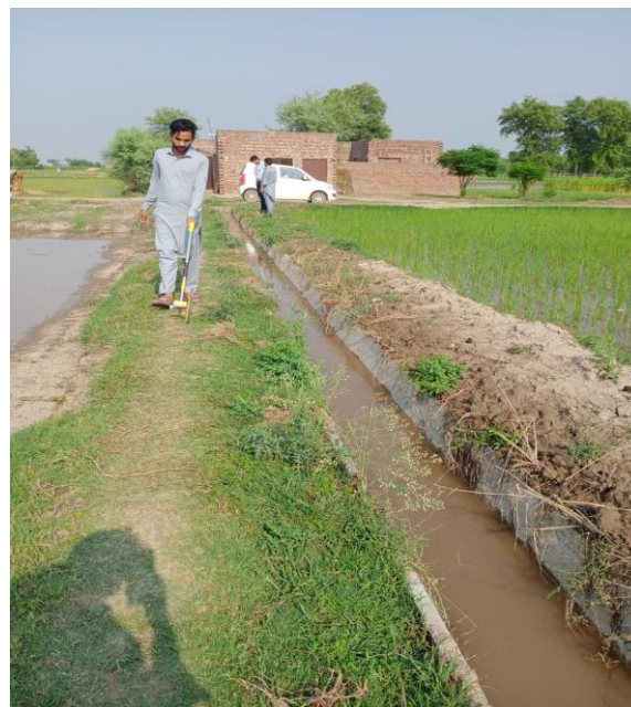
Measuring W/C by measuring wheel W/C No 41350-TL
