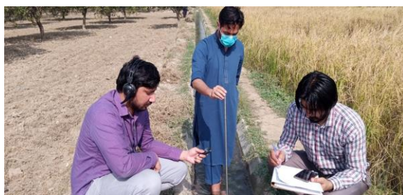
Field Team taking Water Flow Measurement at Watercourse No. 18575-CR Raiwind Lahore
