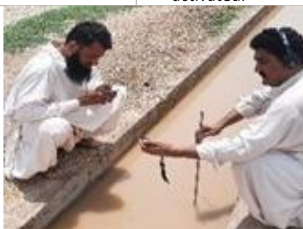
Taking Water Flow Measurement with pigmy meter at WC Shehzad Ahmed
