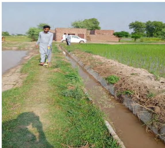
Figure 4.20: Measuring water course length by measuring wheel at Water Course No 41350-TL
