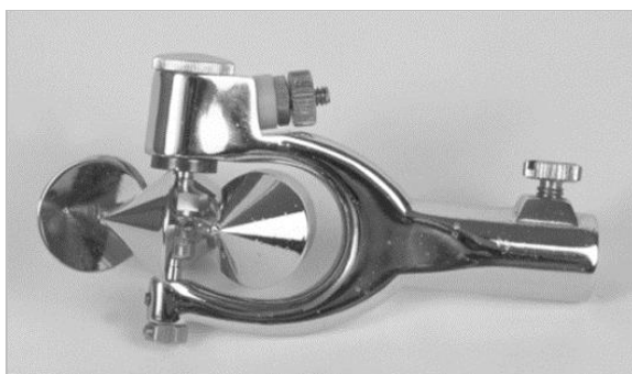
Figure-7.4: Pygmy Current Meter
