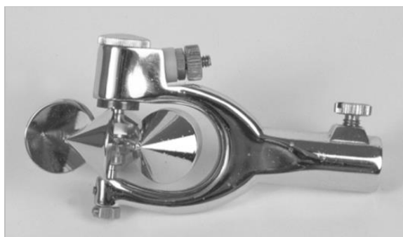
Figure-7.4: Pygmy Current Meter
